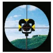
Gone are the days when you had to spend a lot of time aiming at the target to be measured. Today, TPS700 instruments perform this task with automatic target recognition (ATR).
