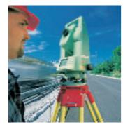
Gone are the times when targets had to be aimed at manually. The TPS 700 performs this and other standard processes with its intelligent software and motorized drives.
