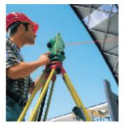
Gone are the times when hard to access targets could only be measured with a lot of effort. Now there are the TPS700 instruments featuring reflectorless distance measurement.
