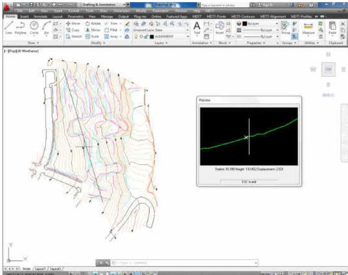
Another interesting command simultaneously draws several profiles on different layers to show the different evolution stages of a terrain.
