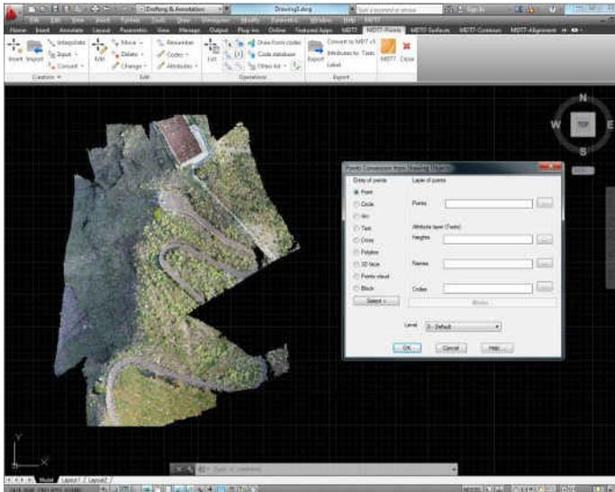
The points may be represented by different shapes and colours on the same drawing. The program will automatically draw the planimetry and the slope change lines, using its code data base on which layers, colours, line types, thicknesses and point code patterns can be defined. Each code can be assigned to a different block for the ground plan, elevation and 3D aiming at a subsequent realistic view.
