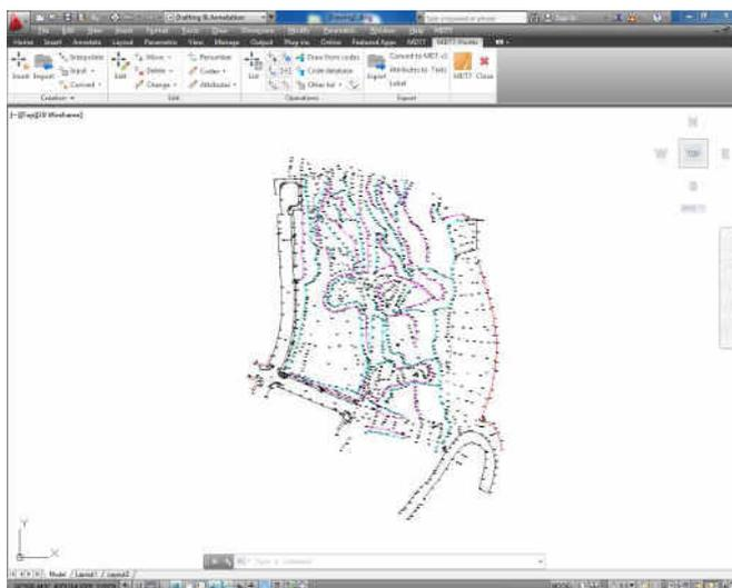
The points are intelligent objects so they can be deleted, moved or changed of layer using conventional commands, or blocks with attributes which makes easier compatibility with other CAD systems or applications.
