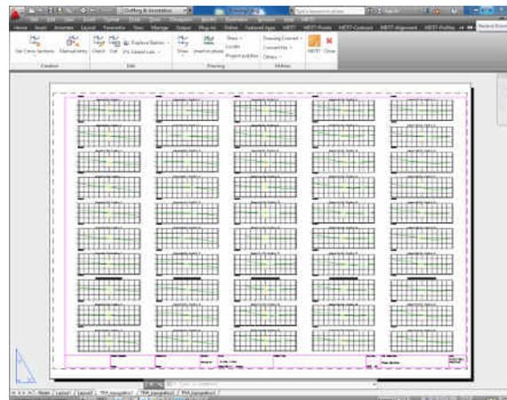
The profiles may be updated automatically when the original alignment or surface have changed. Furthermore, it has a powerful CAD independent profile editor which allows graphic and numerical editing.
