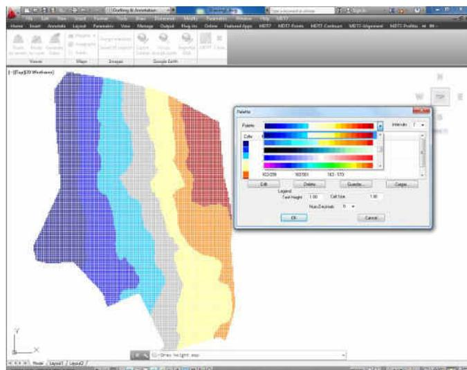
MDT includes a powerful terrain viewer which shows the surface with the textures applied and 3D objects with the possibility of customising the sky and the background. It also has options for measuring 3D distances, obtaining a quick profile, simulate flooding or generating a video based on the tour along a polyline.
