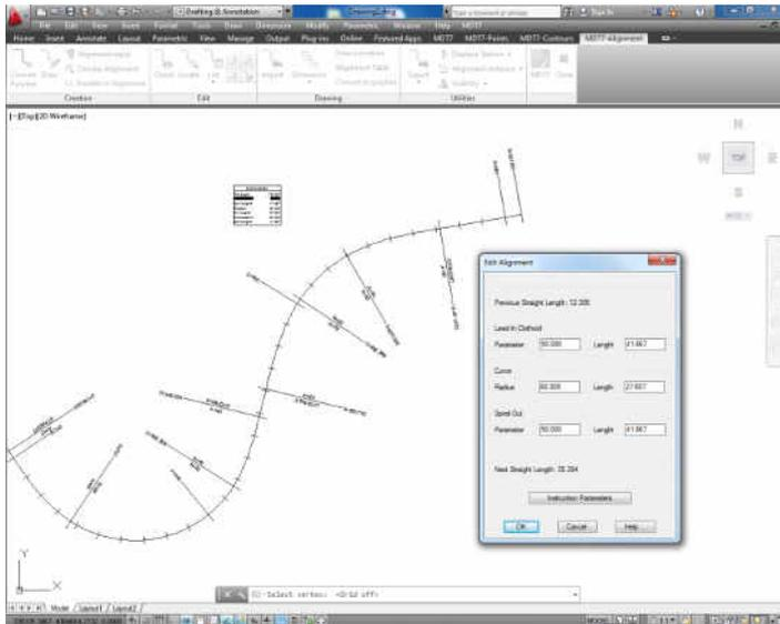
The horizontal alignments which will be used on longitudinal profiles and cross sections may be created interactively by means of lines, circular arc or clothoid segments and also from polylines, numeric input or importing files in the most usual commercial formats.
