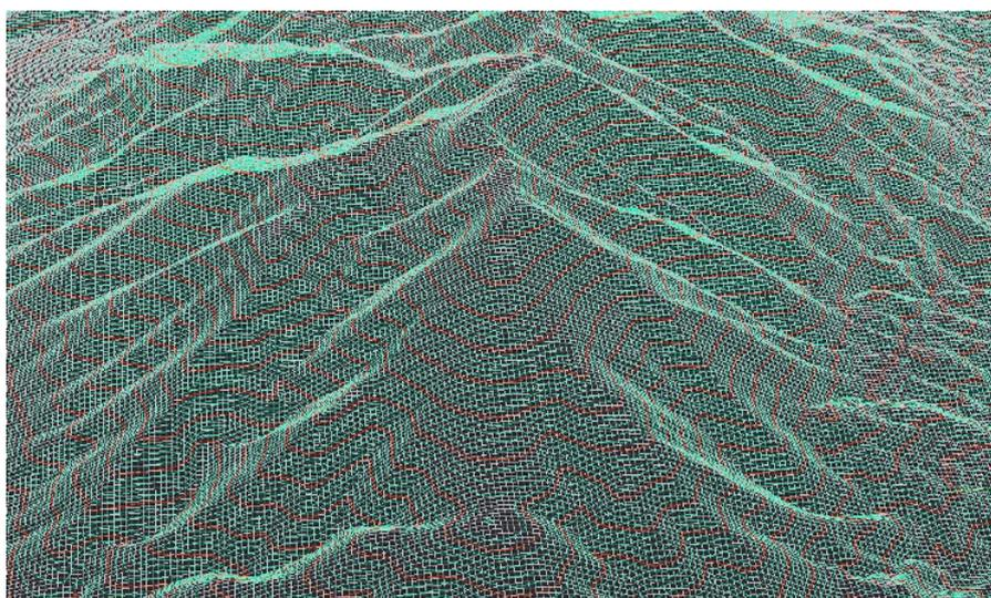
With MDT 7 a mesh can be defined as the present surface and it may be used to identify elevations, quick profile, generation of contours, longitudinal profiles and cross sections etc. This is particularly useful for working simply with terrain data from LIDAR or digital models downloaded from public or private entities.
